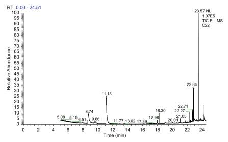
**Figure 1.** Chromatogram for a 5 ppm concentration standard. 1,8-Cineole comes out at 9.62 min and the internal standard, terpinolene, at 11.12 min.
